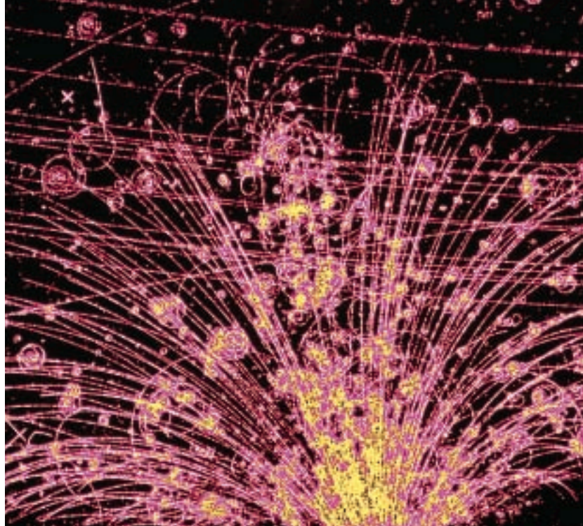
Figure 13 Particles of nuclear radiation can be detected as they leave trails of bubbles in a bubble chamber.
