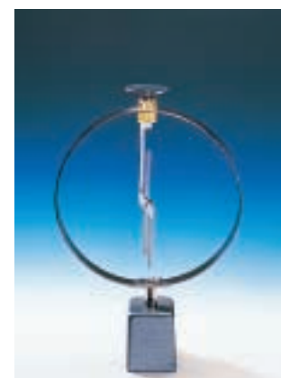
D The electroscope leaves lose their negative charge and come together.
