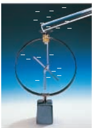
A The electroscope leaves are charged with negative charge.
