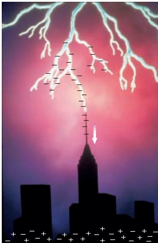
Figure 9 A lightning rod directs the charge from a lightning bolt safely to the ground.
