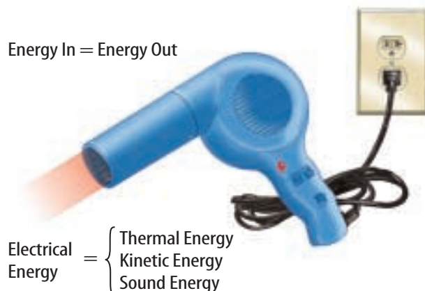
Figure 11 The law of conservation of energy requires that the total amount of energy going into a hair dryer must equal the total amount of energy coming out of the hair dryer.
