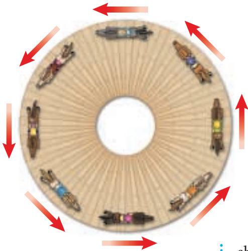
Figure 11 The speed of the horses in this carousel is constant, but the horses are accelerating because their direction is changing constantly.
