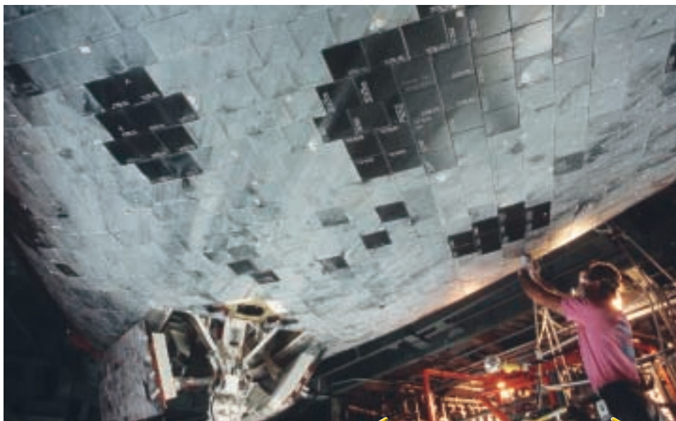
Figure 4 NASA has had an ongoing mission to improve the space shuttle. A technician is replacing tiles damaged upon reentry into Earth's atmosphere.
