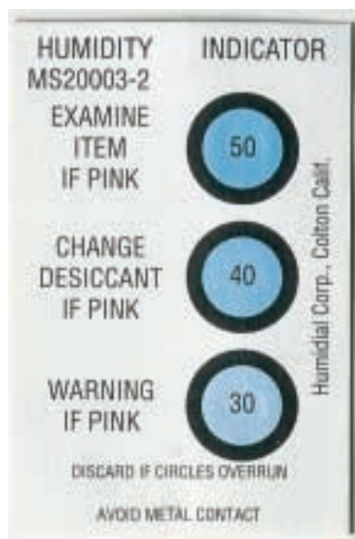
Figure 17 This humidity predictor uses cobalt chloride.
