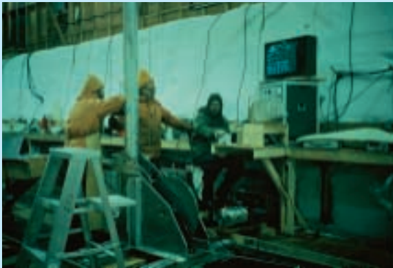
Drilling to the bottom of the Greenland Ice Sheet takes place in a deep trench dug in the snow surface, and uses an electronically controlled drill.
