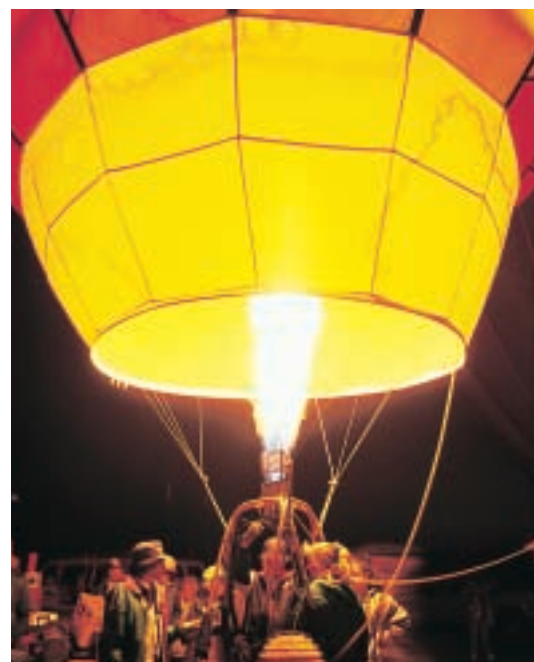
Figure 10 Heating the air in this hot-air balloon causes the particles in the air to separate, creating a lower density inside the balloon.
