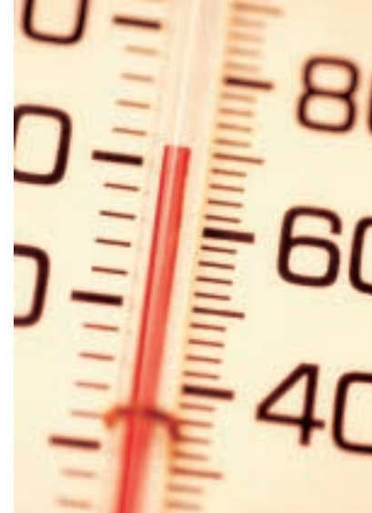
Figure 9 As the thermometer is heated, the column of liquid in the thermometer expands. As the temperature cools, the liquid in the thermometer contracts.
