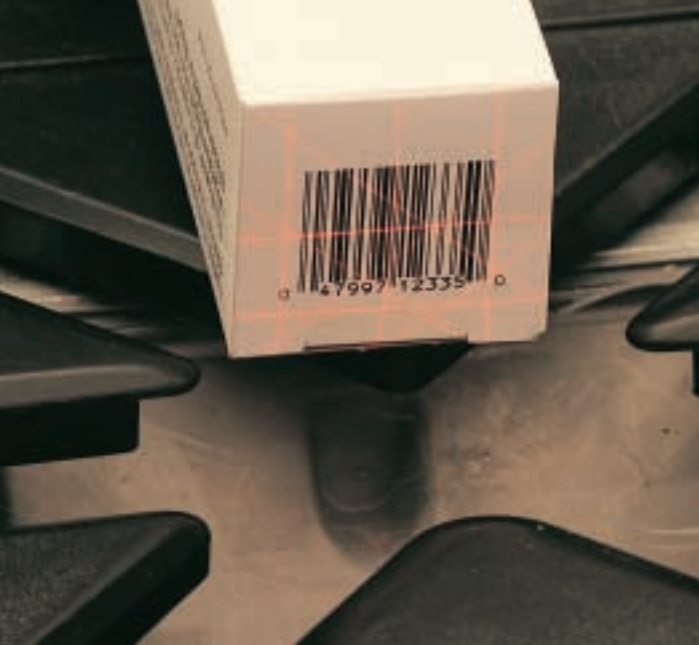
Figure 25 Optical scanners like this one use lasers to find the price of various products.
