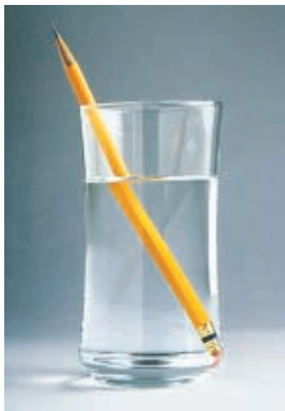
Figure 15 The pencil looks like it is broken at the surface of the water because of refraction. Does light travel faster in water or air?
